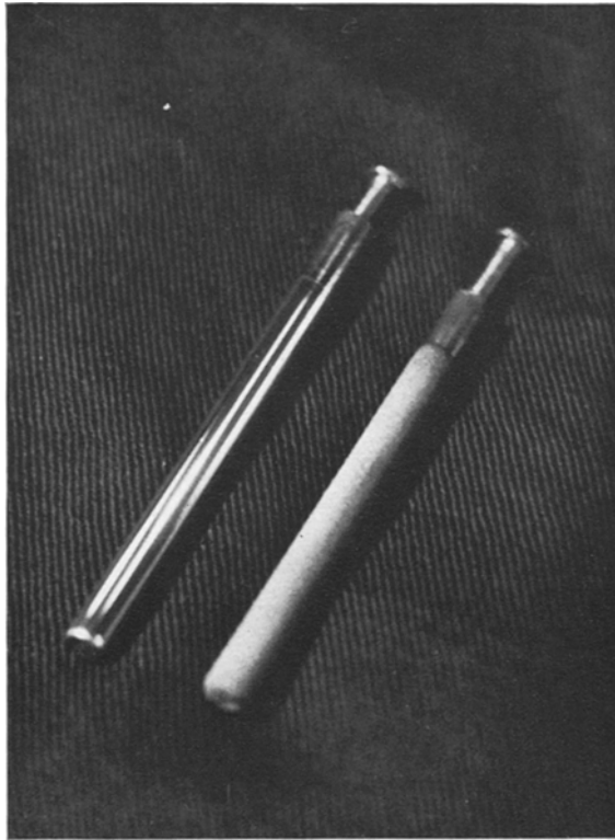
Fig. 1. Specimens plated with (left) and without (right) products of hydrolysis present in the melt.
